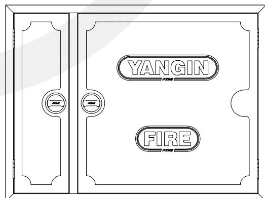
KAPASİTE / CAPACITY : 1" 20m Hortum + 6 kg KKT Yangın Tüpü / 1" 20m Hose + 6 kg DRY Fire Extinguisher
